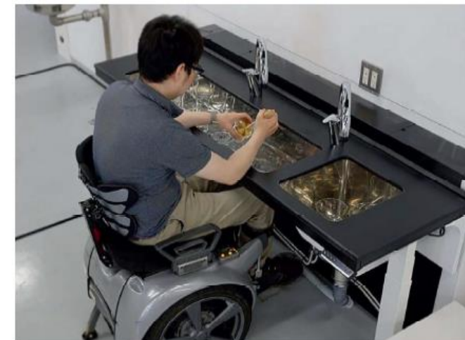
Fig. 1 | Wheelchair-accessible sink from Yamato Scientific Co., Ltd. and GK Sekkei Inc. The sink has several accessible features, including an electrically elevated top panel, leg clearance, a touchless faucet (allowing for use with a shorter reach), a rounded front edge of the sink (to avoid arm pain), an easy-to-grip structure on the inside of the sink, and wider and multiple sink units. Reprinted with permission from ref. 5, Yamato Scientific Co., Ltd.
